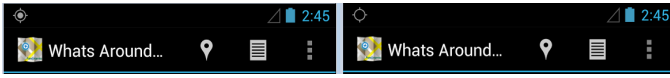
Fig. 1: One version of the existing Android location access disclosure (Google Nexus with Android 4.2.2). On the top left corner, the symbol gets filled and unfilled when the foreground app uses GPS localization. Different versions and vendors of the Android platform have used different kind of symbols, for example, a blinking satellite on the right side of the notification bar. Our research (as anticipated) indicates that this is not an effective disclosure.
